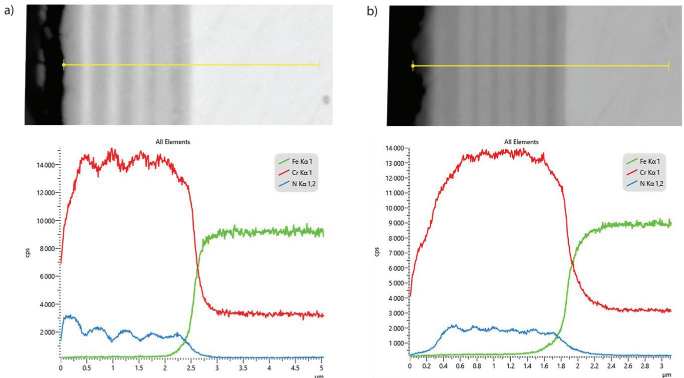
Fig. 4. Linear analysis of the relative concentration of Fe, Cr and N on the cross-section of 10 × Cr/CrN (a) and 14 × Cr/CrN coatings (b)
