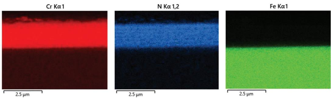
Fig. 3. Elemental mapping of Cr, N and Fe concentration in 14 × Cr/CrN coating
