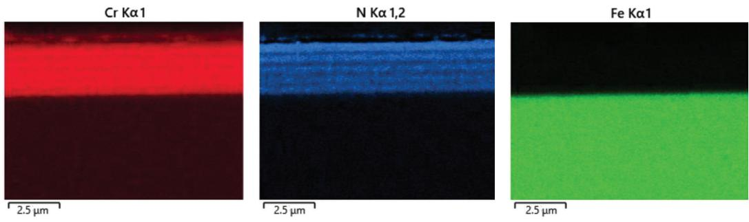
Fig. 2. Elemental mapping of Cr, N and Fe concentration in 10 × Cr/CrN coating
