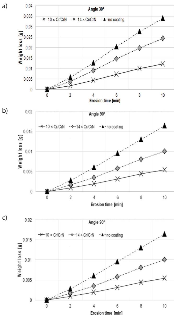
Fig. 6. Weight loss during erosion testing of 10 × Cr/CrN and 14 × Cr/CrN coatings at impact angles of 30° (a), 60° (b), and 90° (c)
