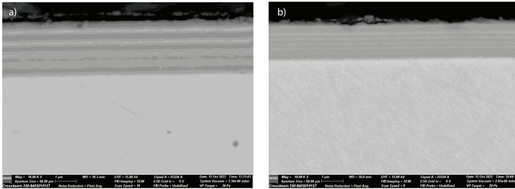
Fig. 1. The microstructure of two types of obtained multilayer Cr/CrN coatings with 10 (a) and 14 sublayers (b)
