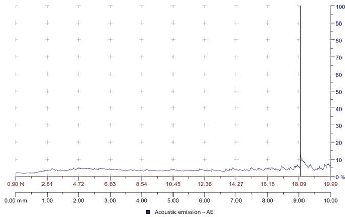
Fig. 5. Acoustic emission graph test for 10 × Cr/CrN coating
