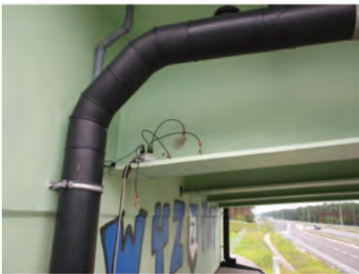
Photo 4. System with thermal sprayed zinc coating, sealant, epoxy coating, polyurethane coating
