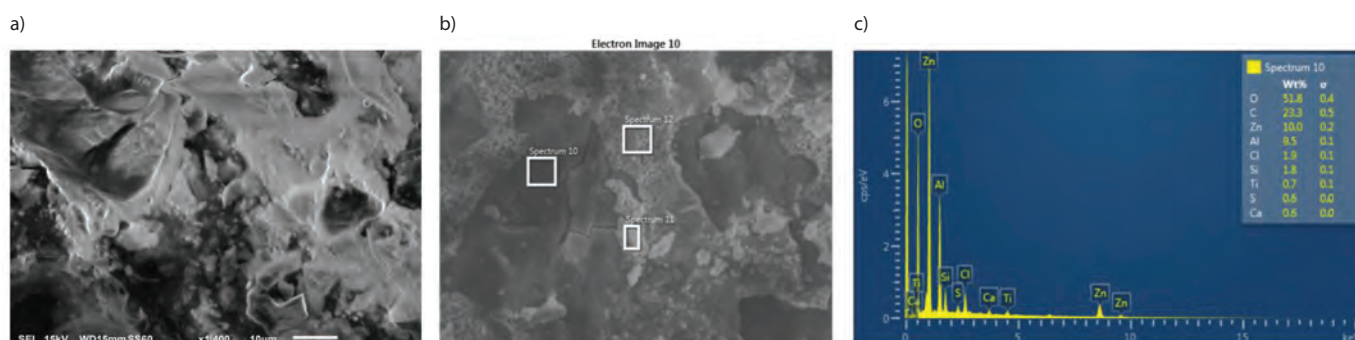
Fig. 2. Structure 2, external surface of the top coat: a) surface appearance at \times 1,400 magnification b) chemical composition analysis sites, c) chemical composition histogram of site 10
