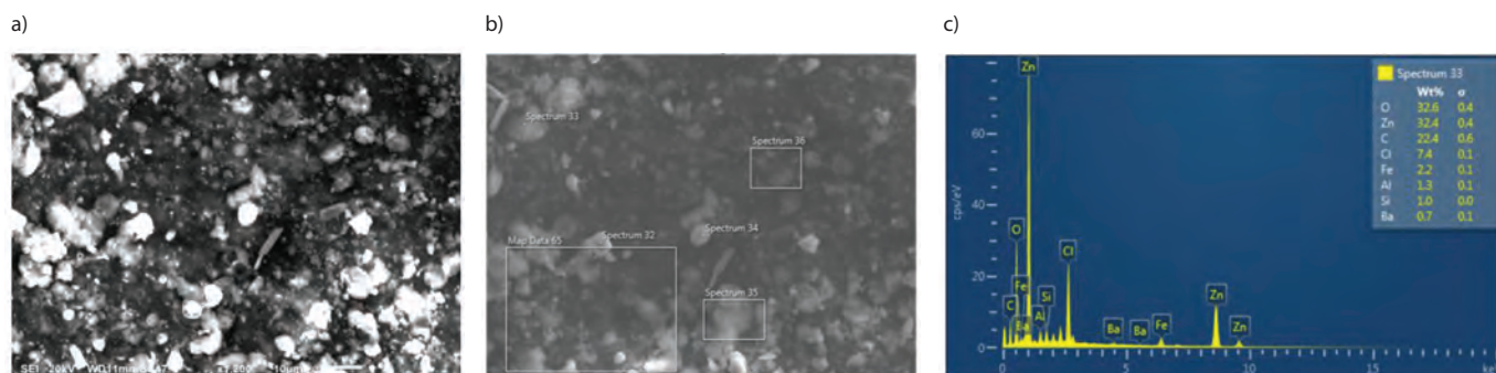
Fig. 1. Structure 1, external surface of the top coat: a) surface appearance at \times 1,200 magnification, b) chemical composition analysis sites, c) chemical composition histogram of site 33
