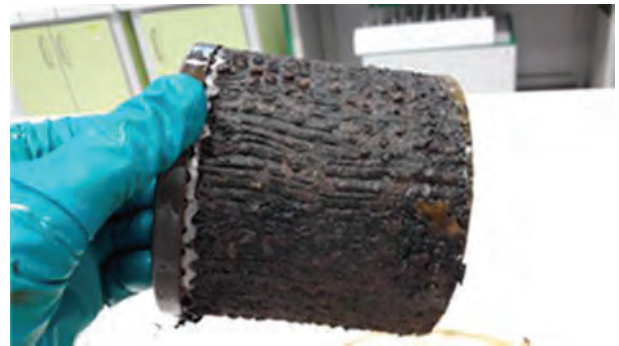
Photo 2. Photograph of clogged fuel filter Source: [38, p. 5].
