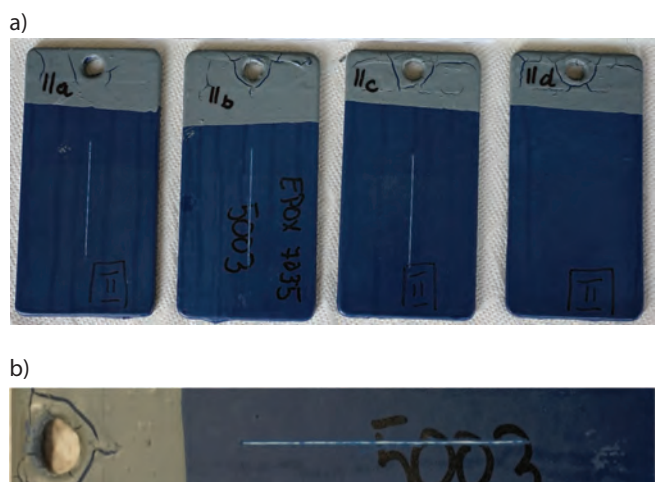
Fig. 6. Surface of the samples protected according to variant C after 1,440 hours of exposure in the salt chamber: a) set of samples, b) artificial damage to the corrosion protection system
