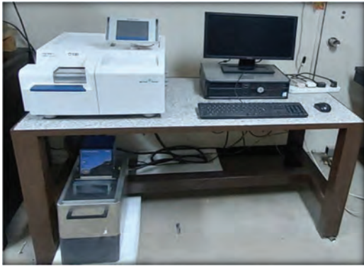
Fig. 6. The thermogravimetric analysis device
