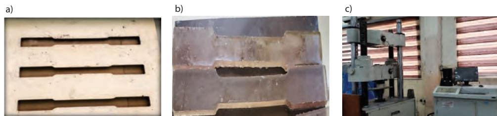
Fig. 4. Tensile strength test: a) mold used to prepare the samples, b) shape of the samples used for measurement, c) the device used to measure tensile strength
