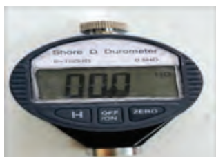
Fig. 3. The device Shore D used to measure hardness
