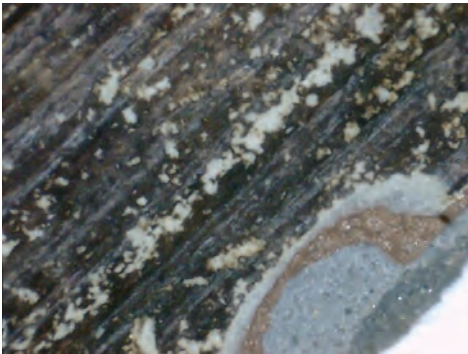
Photo 8. Damages and unevenness of coatings (from the top) in the vertical axis of the paintings – photo taken with a metallographic microscope
